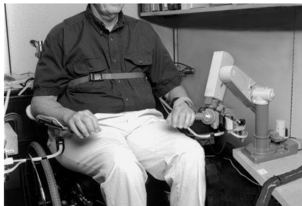
Figure 16.1 Mirror-Image Motion Enabler, MIME (Burgar et al., 2000)
